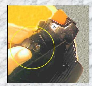
Other handles on the front cover are removed the same way, first remove the screw covers then undo the securing screws.
