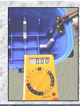
The reed switch is glued to the front cover with contact cement.
