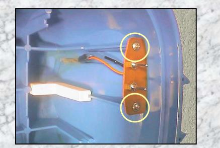
When gluing the switch back into position be sure to test its position with the multimeter before finally gluing. If incorrectly positioned it is possible for the reed switch to be 'on' permanently and only turned off by depressing the button.
